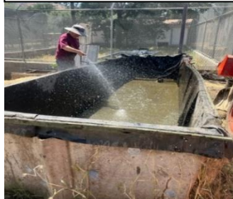
Dirty, sludge filled biofilter
